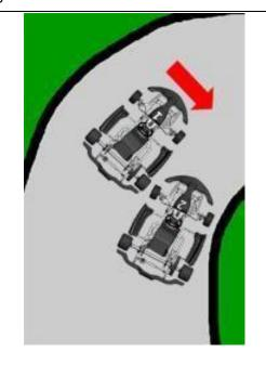
**EDGE-INTO** means that Kart 2 drives next to Kart 1 (e.g. in order to start an overtaking action) without possessing enough drivable section (including kerbs). It is irrelevant if Kart 2 is completely or partially next to Kart 1 or if Kart 2 is completely or partially off the track.
